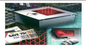
Shop and Go in Safeways allows the customer with ABC cards to use handscanners, ("Handiscan") themselves to scan the bar codes of the items. To get a handscanner the ABC card has to be placed into a card receiver slot. A light then flashes to indicate the handscanner to take from the rack.
