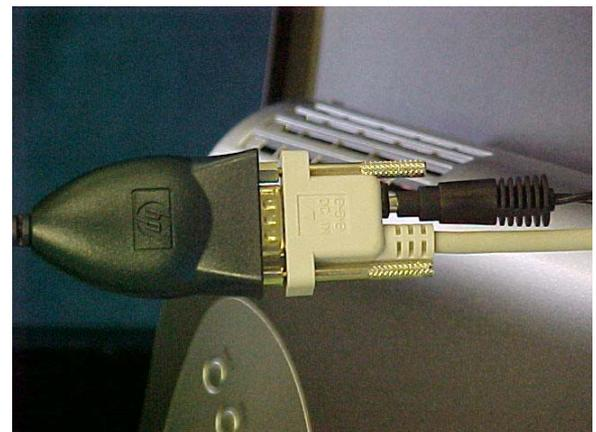
5. The network connection adapter plugs into the side of the laptop.
